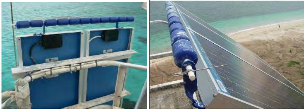
Figure 2. Adding cones to flat lantern surfaces
